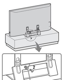
**1** Install a wood screw (4 mm in diameter, not supplied) in the monitor stand.
